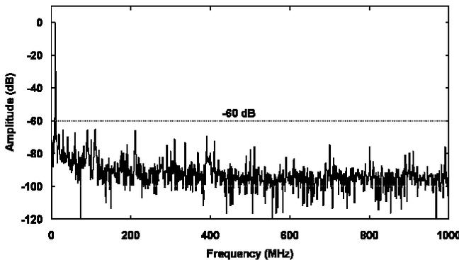
Fig. 14: FFT on a single 10-MHz 0.8-V<sub>p-p</sub> sine wave acquisition.
