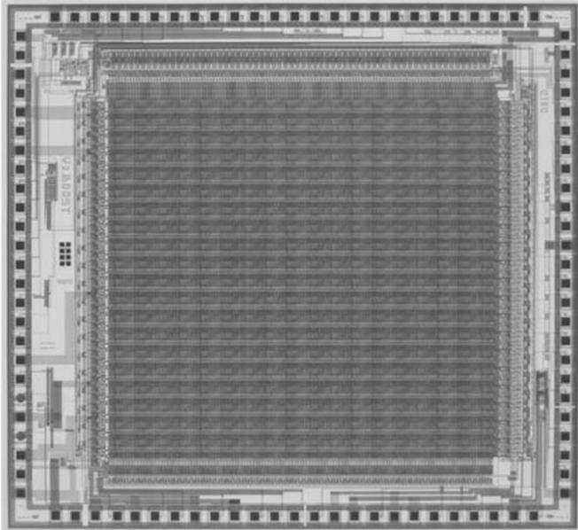
Fig. 3: The MATAcq chip layout. It contains 100,000 transistors on a 30 mm<sup>2</sup> silicon die. The 2560-cell switched capacitor array covers 80% of the chip area.
