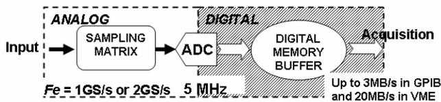
Fig. 6: Data flow in the MATACQVME board.
