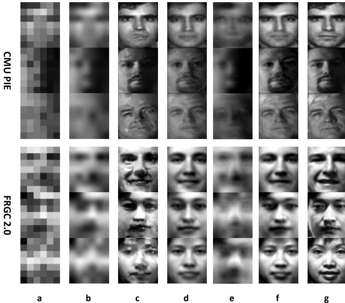
Figure 3. SR results: (a)input VLR images (7 x 6), (b) SR results by Bicubic interpolation,(c) by Hallucination Face method (HF)[1], (d) Eigentransformation based Face SR method (EF) [18], (e) KPCA-based Face SR method (KF) [2], (f) Our proposed method (RL), (g) original HR images. The resolution of reconstructed HR images is 56 x 48.
