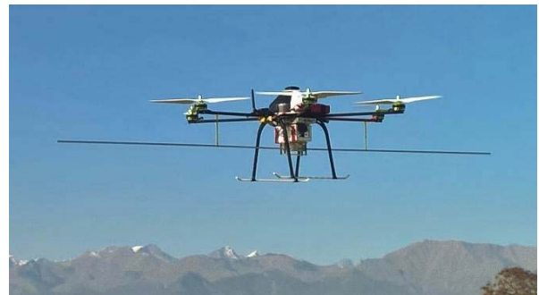
Fig. 1. The flying test source consisting of the UAV equipped with the RF transmitter and the dipole antenna operating at 50 MHz.
