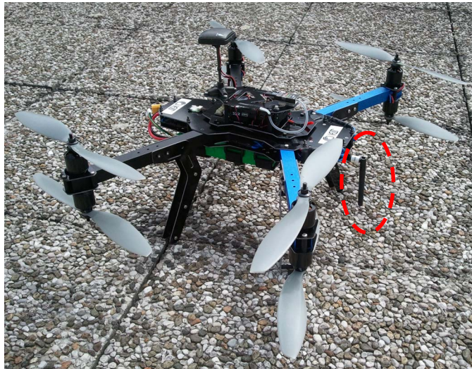
Fig. 8. Antenna Under Test (red dashed contour) mounted on a commercial micro UAV (3DR X8+).
