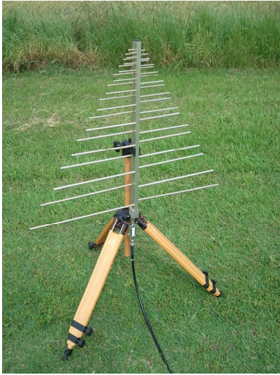
Fig. 7. The log-periodic antenna used as a known reference for the characterization of the telemetry monopole onboard the UAV.
