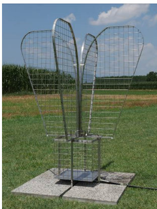
Fig. 4. The dual-polarized Vivaldi antenna on the measurement field.
