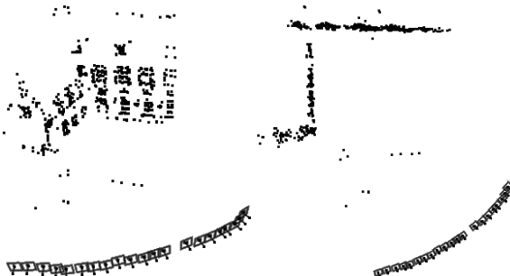
Fig. 5. Castle: Computed cameras and 3D point structure. The plan view shows the accuracy of the self calibration.
