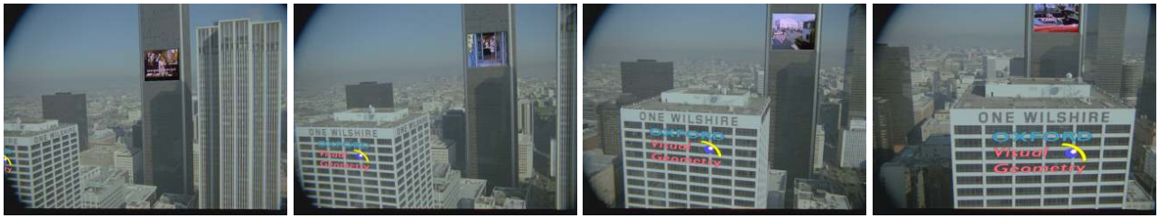
Fig. 8. Wilshire : Augmented reality. Planar surfaces are identified in 3D, then 2D homographies are computed which map the augmenting images onto the planes. Note that images appear to be rigidly attached onto two skyscrapers.
