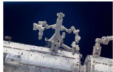
Figure 7. The Special Purpose Dexterous Manipulator on ISS.
