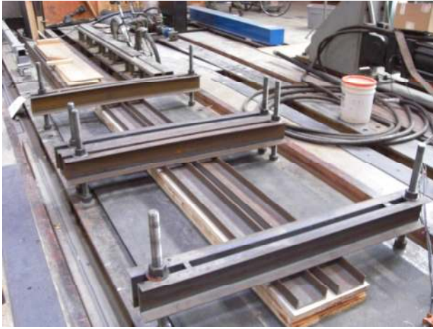
Figure 1: Fixture for pressing CLT panels
