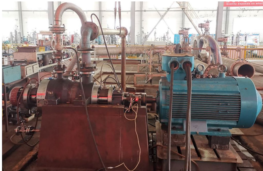
Figure 7. Centrifugal pump test platform.
