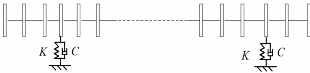
Fig. 7. Transfer matrix model of bearing-rotor system.
