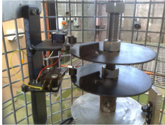
Figure 3.2 A photo of control mechanism to enable reversible rotation.
