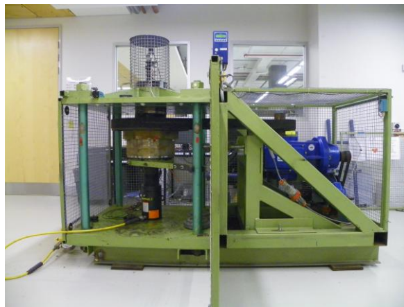
Figure 3.1 A photo of slew bearing laboratory test rig.
