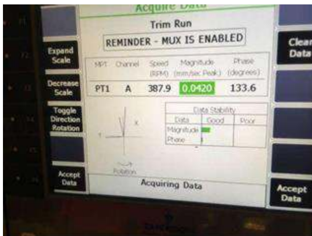
Fig. 26. Acquiring final trim run data
