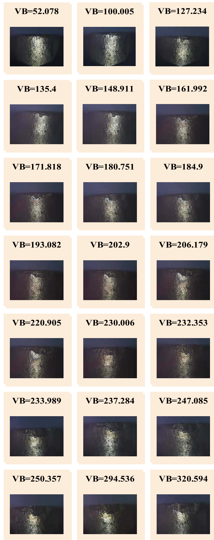
Figure 4. Wear Morphology from test of the cutting insert.
