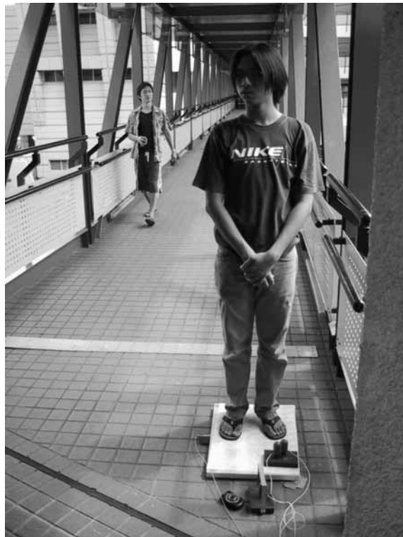
Fig. 10. Measurement of mitigating effect of stationary occupant on walking-induced response.
