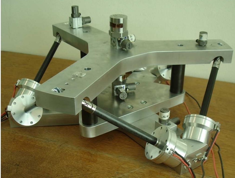
Figure 10: View of the isolator.
