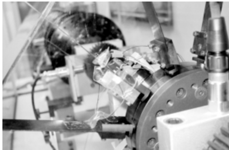
Fig. 27. Photograph of the blade-PZT root holder.
