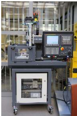
Fig. 5. 3-Axis vertical CNC machine that is used to carry out this paper
