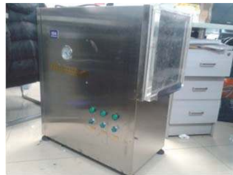
FIGURE 14: Vacuum deaeration tank.
