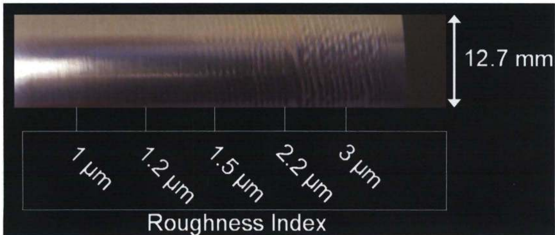
Figure 10. Surface Roughness Performance (1200rpm, 127 µm/rev feed)
