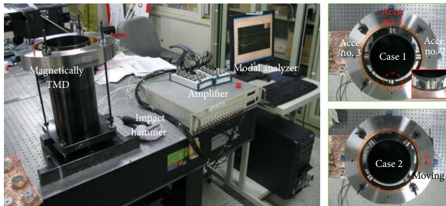
FIGURE 15: Experimental setup of mTMD and arrangements of magnets.
