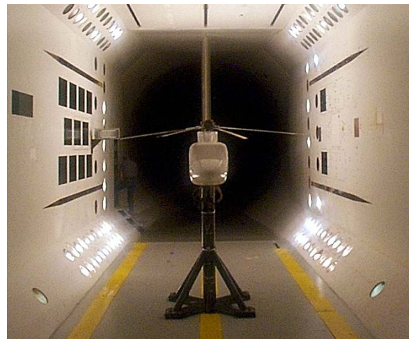
Figure 3. The ARES testbed in the TDT with the ATR hardware installed.
