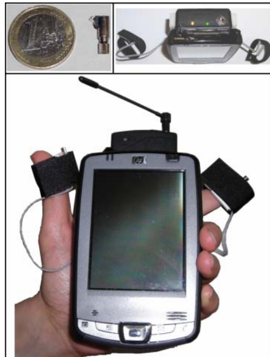
Figure 1. From the top left-hand corner: one of the actuators used in the experiment, the PDA fitted with the RFID reader and the haptic module, and how the device fits on the user's hand.
