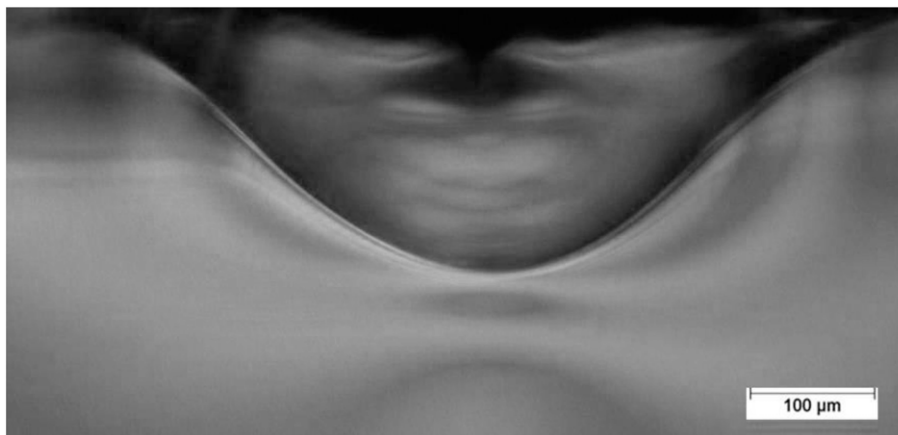
FIGURE 10 | View through a polished edge showing the extent of subsurface deformation for a 170 kgf dynamic Vickers indent in ion-exchanged damage-resistant glass. The impact velocity was 1,005 mm/s and the contact event time was 512 \mu\text{s} .
