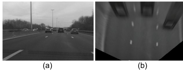
Figure 2 Transformation to the rectified domain through IPM. As opposed to the original image (a), in the rectified image (b) the effect of perspective is removed and thus motion of vehicles is easier to model.
