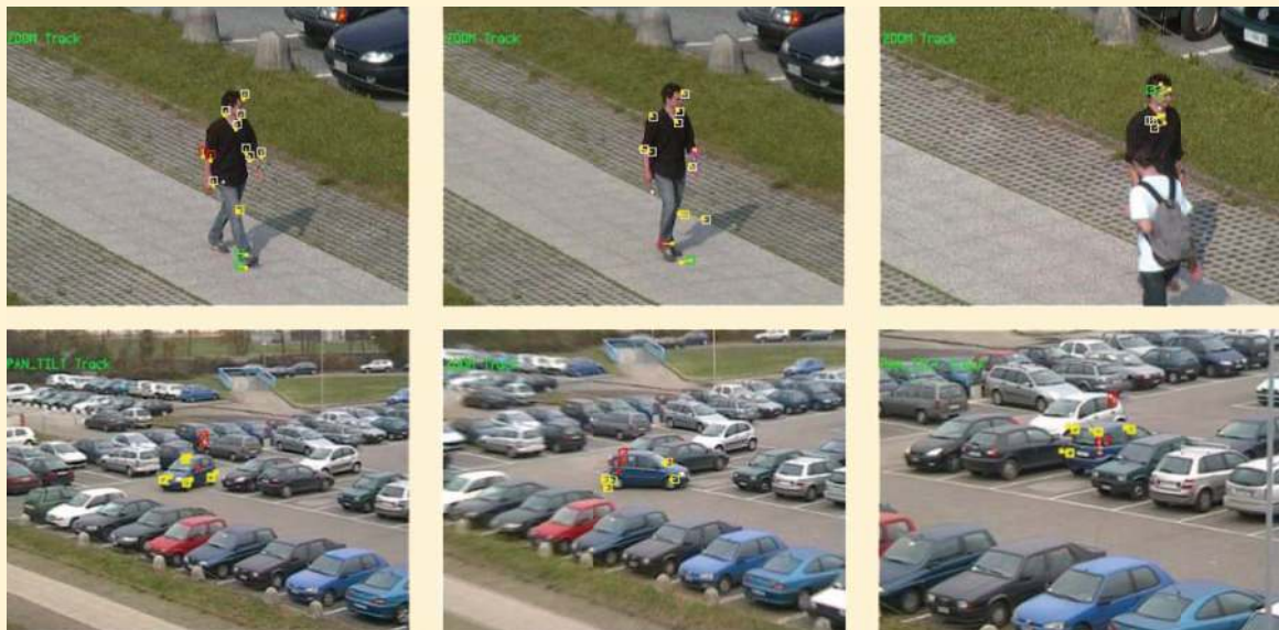
[FIG3] Sample frames of two test sequences used for evaluating the active tracking of nonrigid and rigid objects. The small boxes represent the tracked feature points organized in clusters depending on their color. The red dot represents the computed fixation point on the selected cluster (white for nonrigid object and yellow for rigid object).
