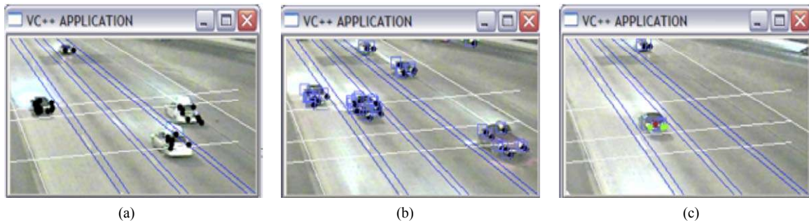
Figure 2. Detected Harris-Stephen corner interest points on vehicles.
