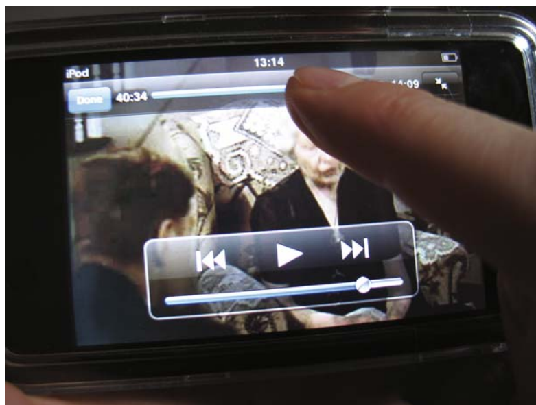
Figure 1. The iPod touch's video player (iPod touch ver. 1.1.4). Users can skip scenes using two buttons and navigate through the file along the timeline using a slider at the top of the window. Browsing granularity is high due to the small size of the screen, thus preventing users from performing detailed browsing and exact positioning.
