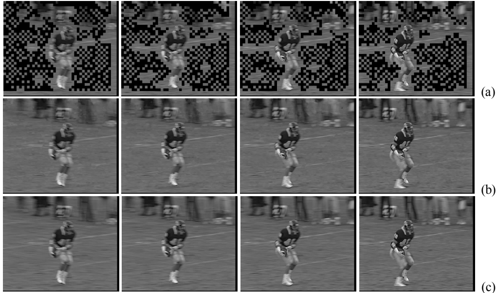
Fig. 4. Four B-pictures in one GOP of sequence “Football”: (a) original frames with removing masks (shaded blocks indicate motion-aligned removed ones), (b) reconstructions of our scheme with QP=18, (c) reconstructions of H.264/AVC with QP=18.
