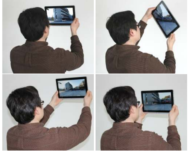
Figure 2: Top : The tablet interface is free to rotate along all axes in space to provide a virtual window. Bottom : Front camera face tracking provides zoom control.
