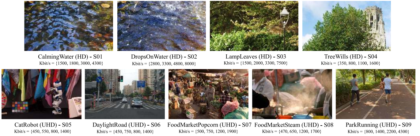
Fig. 3. Test sequences and target bitrates used for experimental results: proposed for the Grand Challenge on Video Compression Technology at ICIP 2017. All sequences are 60 fps except for ParkRunning which is 50 fps.
