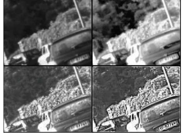
FIGURE 3: Single frame from Sequence 2: input frame (upper left), histogram equalization (upper right), our algorithm (bottom left), simulation of the hardware implementation of our algorithm (bottom right). Notice that our algorithm yields a better visual quality than a simple global operator as histogram equalization. In particular, the details are better rendered, and this is true even with the simplified version for the hardware implementation.
