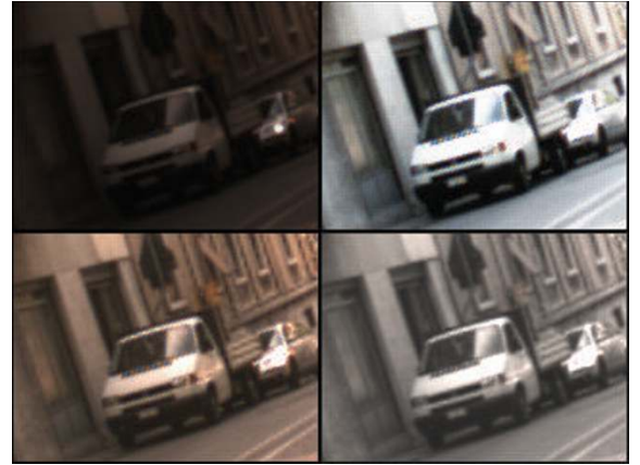
FIGURE 4: Single frame from Sequence 2, color results: input frame (upper left), histogram equalization (upper right), our algorithm in RGB (bottom left), our algorithm in YCbCr (bottom right).
