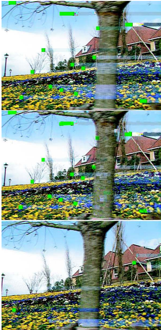
FIGURE 8: Three frames using Early Resynchronization only. (Note: to highlight the location of the errors, no spatial concealment used.) Top is the first I-frame of the sequence. Middle is the second frame (B-frame). Bottom is the next I-frame (seventh frame in this sequence).
