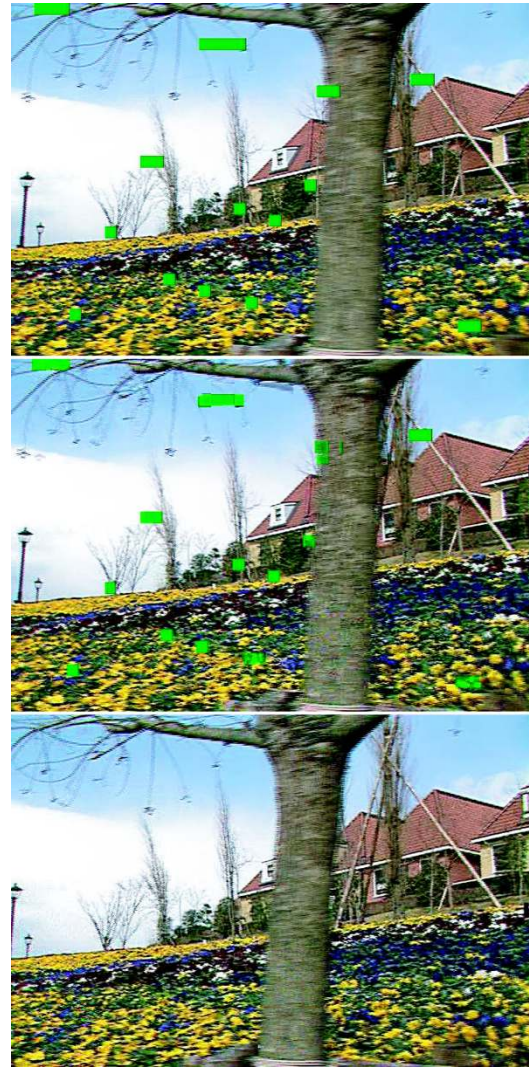
FIGURE 9: The results of the Steganocodec, with same error sequence as before. Again no spatial error concealment. Top is first frame (I-frame) of sequence. Middle is second (B-frame), and bottom is next I-frame in sequence. Note the importance of recovering the DCT-DC values.
