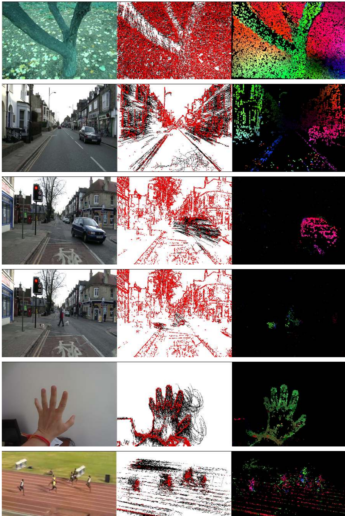
Fig. 8 From left to right: the input video, the particles (in red) and their trajectories (in black), and the semi dense motion field, using polar coordinates of the velocity vector as (hue, intensity) colour code.
