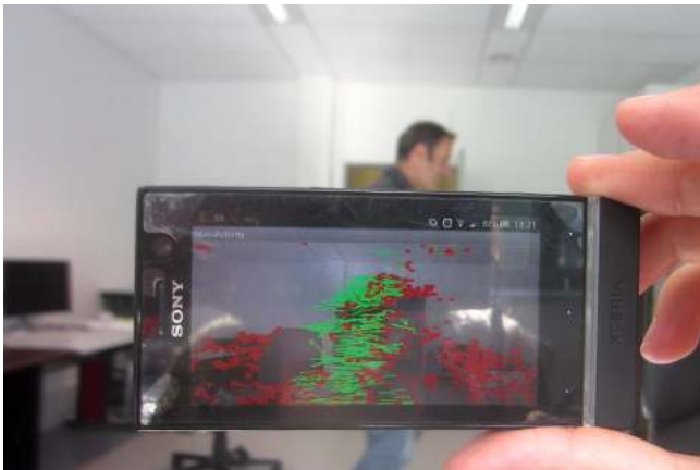
Fig. 9 The tracker running at 10Hz on a low-end Xperia U smart phone embedding an ARM dual-core STE U8500.
