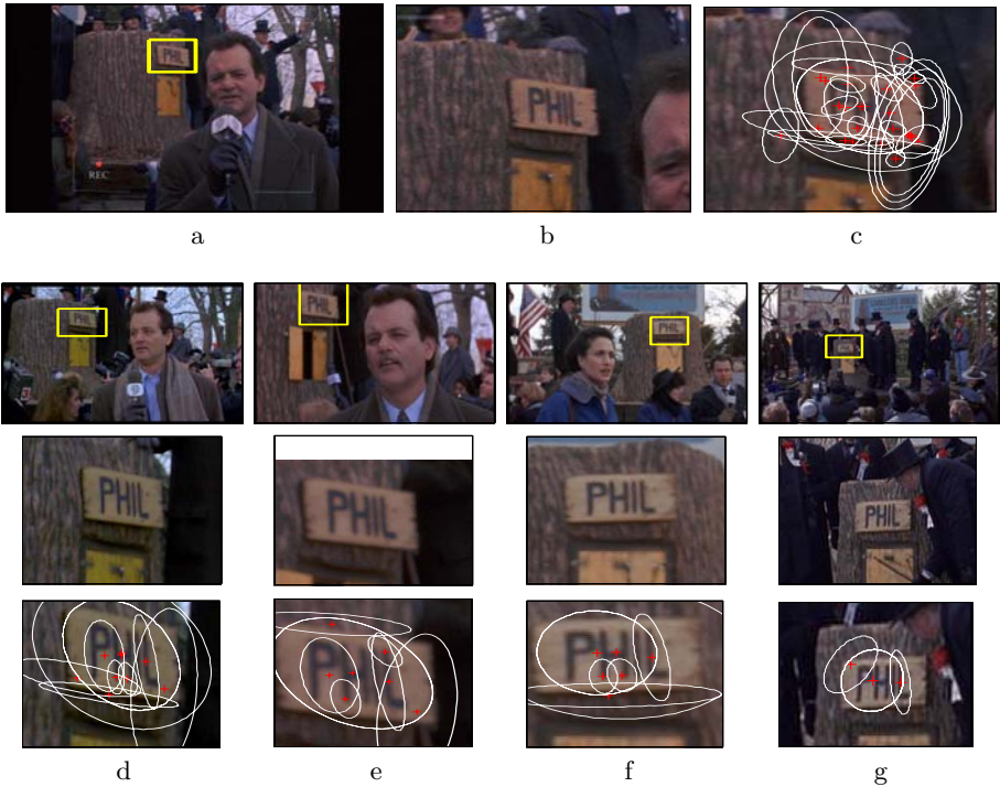
Fig. 8. Object query example II: Groundhog Day. (a) Keyframe with user specified query region in yellow (phil sign), (b) close-up of the query region and (c) close-up with affine covariant regions superimposed. (d-g) (first row) keyframes from the 1st, 4th, 10th, and 19th retrieved shots with the identified region of interest shown in yellow, (second row) a close-up of the image, and (third row) a close-up of the image with matched elliptical regions superimposed. The first false positive is ranked 21st. The precision-recall graph for this query is shown in figure 7 (object 5). Querying 5,640 keyframes took 0.64 seconds.
