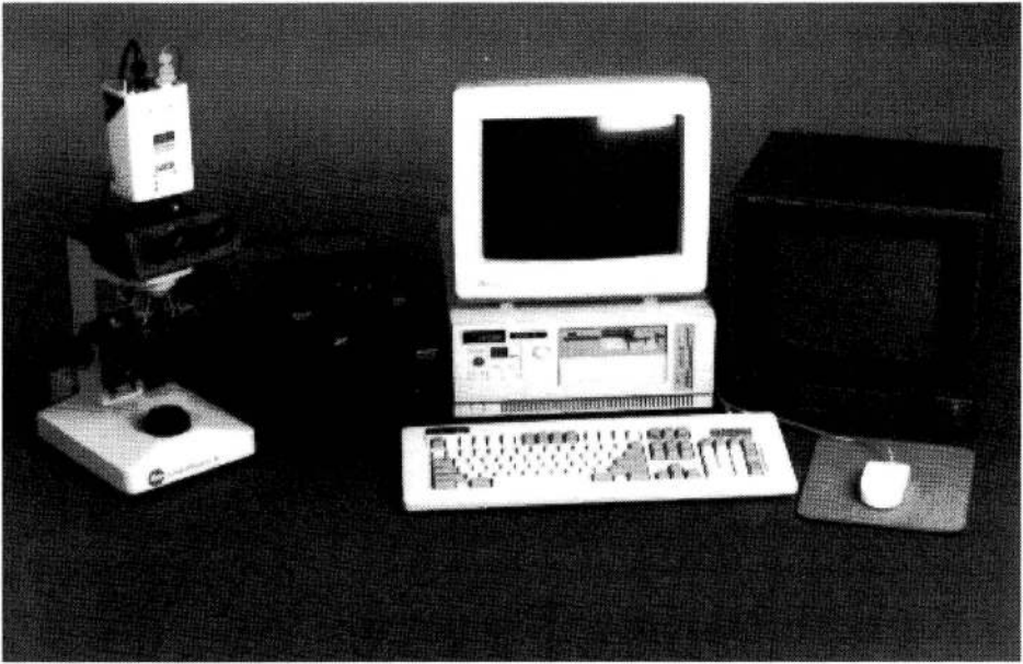
Figure 1. A typical VIA system, comprising microscope with video camera, computer with installed digitiser card and VIA software, plus video monitors. One monitor is used to view the usual computer output for the selection of appropriate programs and sub-routines, the other to display and manipulate the images. In some systems a single monitor suffices. Also shown is a "mouse", used here as a pointer and screen image editing device in addition to the usual computer functions and a video-photographic unit to capture screen images onto film.
