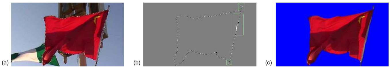
Figure 7: Clip #2, frame 27. (a) 3D graph cut result is shown by the overlaid dashed line. The flag is a rapidly deforming object, but 3D graph cut can capture the shape very well. (b) Dashed lines indicate the boundaries after both the local refinement and overriding operations. The white pixels record the actions of foreground brushing and the black pixels for background brushing. (c) coherence matting result pasted on a blue screen.
