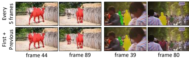
Figure 6: Visual comparisons of the results with and without using the intermediate frame memories.
