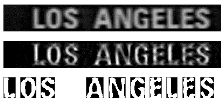
Figure 12: Result of extraction for Gothic font characters. Sub-pixel interpolated and multi-frame integrated image (top). Character extraction filter (middle). Character segments in binary image (bottom).
