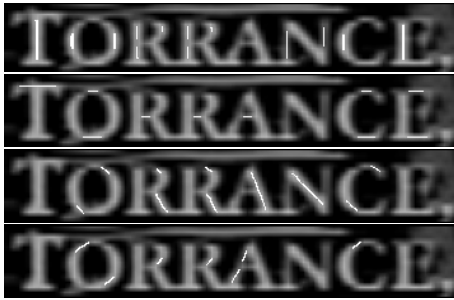
Figure 4: Learning data of filters (white pixels). vertical / horizontal / left diagonal / right diagonal.
