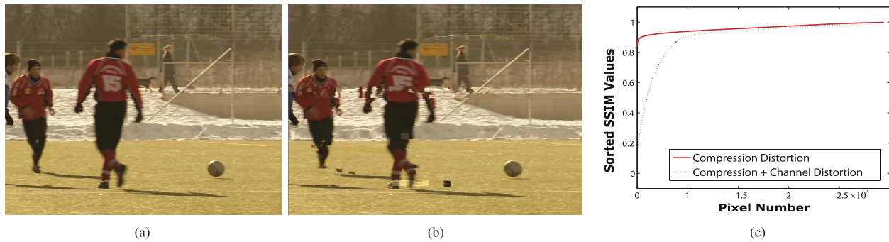
Fig. 2. Comparison of the distribution of local spatio-temporal quality scores for different distortion types. (a) Compression distortion only. (b) Compression and distortions due to errors in communication channel. (c) Curve showing the local spatio-temporal SSIM scores of (a) and (b) sorted in ascending order.
