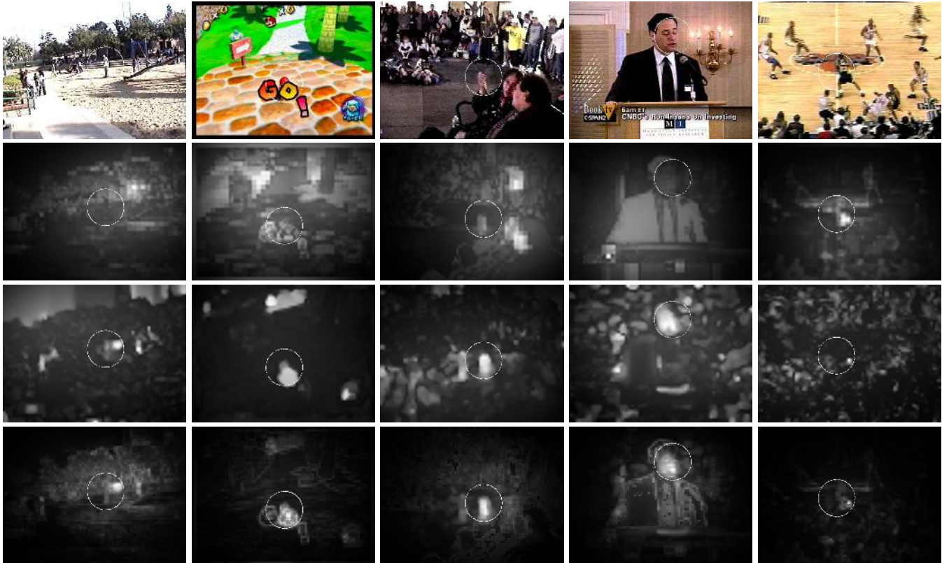
Fig. 7. Visual comparison of spatial, temporal, and spatiotemporal saliency. Row 1: video frames with human fixation point marked with circles; Rows 2 - 4: spatial, temporal, and spatiotemporal saliency maps, respectively.
