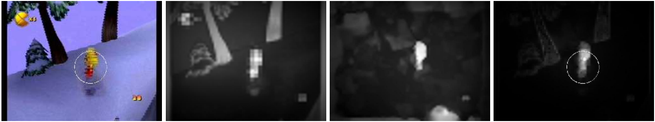
Fig. 4. Sample saliency maps. Column 1: original video frame with human fixation point marked with a circle; Column 2 - 4: spatial, temporal, and overall saliency maps, respectively.
