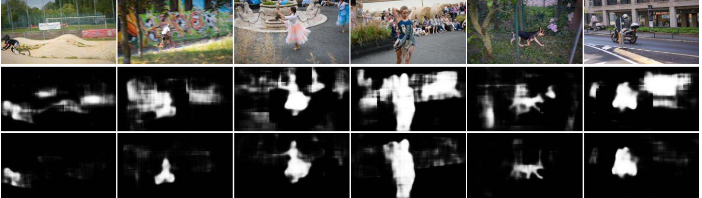
Fig. 8. Qualitative comparison between our static saliency results and final spatiotemporal saliency results. From top to bottom: input frame images, saliency results via our static saliency network, and spatiotemporal saliency results via our whole video saliency model.
