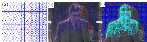
Figure 1. Segmentation by tracing discontinuities. (a) A trajectory spectral embedding has varying density, depending on the scale and kinematic nature of the objects captured by the embedded trajectories. (b) Density discontinuities (shown in red) between spatially neighboring trajectories are strong indications of object boundaries. (c) Video segmentation by discontinuity thresholding.
