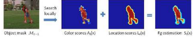
Figure 3. Estimated object location R_t . Given the object mask \mathcal{M}_{t-1} marked as the red contour, we search for a local region in the current frame t and compute the foreground scores based on color and location. The estimated foreground region is used for label assignment.
