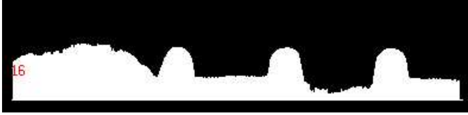
Figure 6: Results of subtracting frame i from frame i+20 , after motion compensation. In the first frames there is large object motion. The three “humps” correspond to smooth cuts
