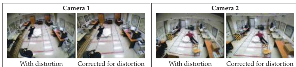
Fig. 15. Examples of images from the two viewpoints before and after distortion correction.
