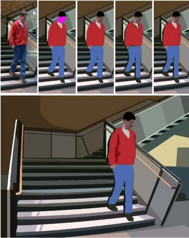
Figure 12: Construction of the final frame. Top row from left to right: original frame, regions as solid shapes, head rendered with segmentation result, edges on all region boundaries, edges only at important boundaries based on edge importance for each region. Bottom image: final frame that now includes subregions within the shirt to show shadowing.
