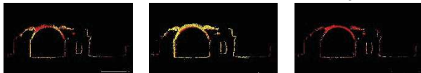
Figure 7. Visual comparison of profiles (A-A' and B-B') extracted on the videogrammetry (red) and ground truth (yellow) point clouds for the employed frame selection methods.
