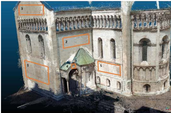
Figure 4. Locations of the five areas used to calculate the plane fitting RMSE useful to evaluate geometric performances of the video-based 3D reconstruction.
