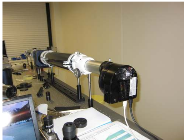
Fig. 8. Optical system compound by the two telescopes used for obtaining a measure of the resolution.
