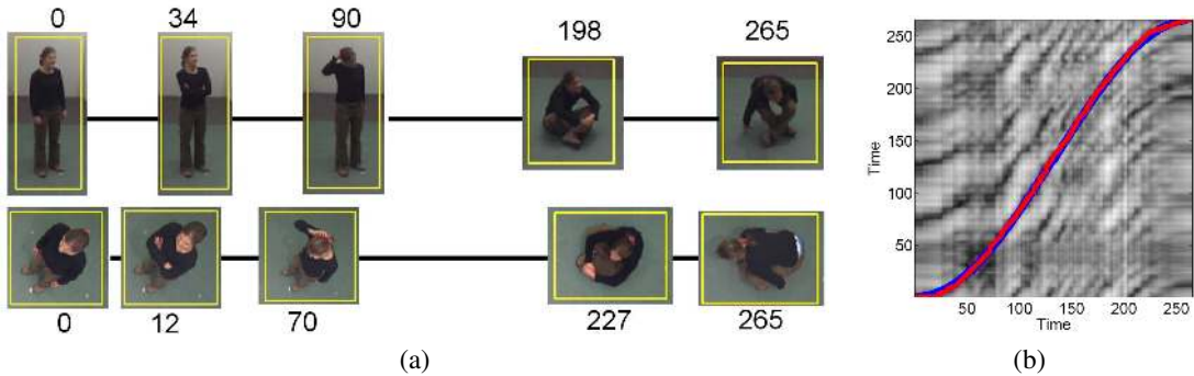
Fig. 7. Temporal alignment of same action performances in videos from different viewpoints and with synthetic de-synchronization. (a): Two de-synchronized sequences with the side and the top views of the same action are represented with a set of matching key-frames. The second sequence has been time warped according to t' = a \cos(bt) transformation. (b): Distance matrix between sequences H(\mathcal{I}^1) and H(\mathcal{I}^2) of SSM-pos descriptors (bright colors represent large distance values). Dynamic Programming (red curve) finds the minimum cost monotonic path from (0, 0) to (T, T) in this matrix. This path coincides almost perfectly with the original warping (blue curve) despite drastic view variations.
