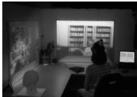
Figure 1. A user in Chapel Hill wearing polarized glasses and an optical tracker communicates with two remote users from Philadelphia (left) and Armonk (right). The stereoscopically displayed remote 3D-scenes are composed from incoming streams of textured 3D data depicting the users, and off-line acquired static backgrounds.
