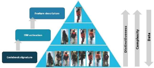
Figure 2. Overview of the three-staged ISM re-identification approach.
