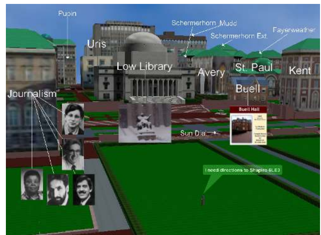
Figure 10. Annotations associated with multiple objects, including buildings and avatar for outdoor user. Building annotations were specified to have higher priority than avatar's annotation, causing avatar's annotation to avoid buildings and their annotations.
