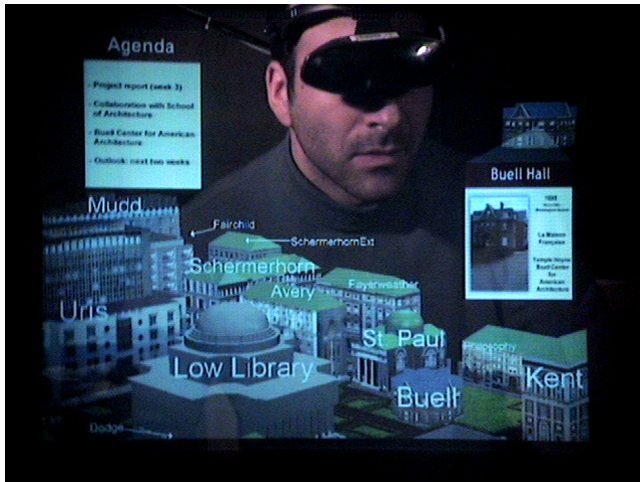
Figure 1. View management in augmented reality testbed (imaged through a tracked, see-through, head-worn display).
