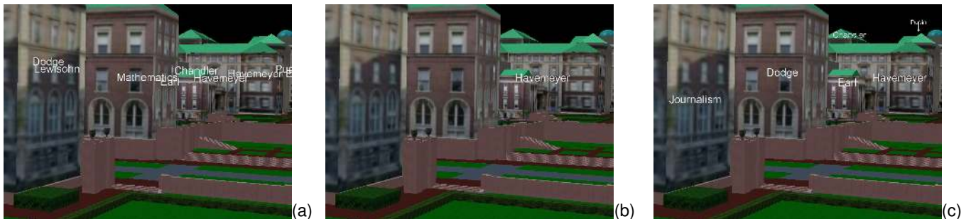
Figure 7. Area feature labeling comparison. (a) Naïve label placement at projected centroid of each building causes overlaps, and mislabeling because of buildings hidden partially or entirely. (b) Suppression of labels for buildings whose projected centroid is not visible. (c) Label placement using approach of Section 4.3.
